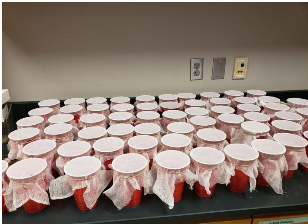
Figure 4.4 Plastic cups covered with cheese cloth and secured with a rubber band.
