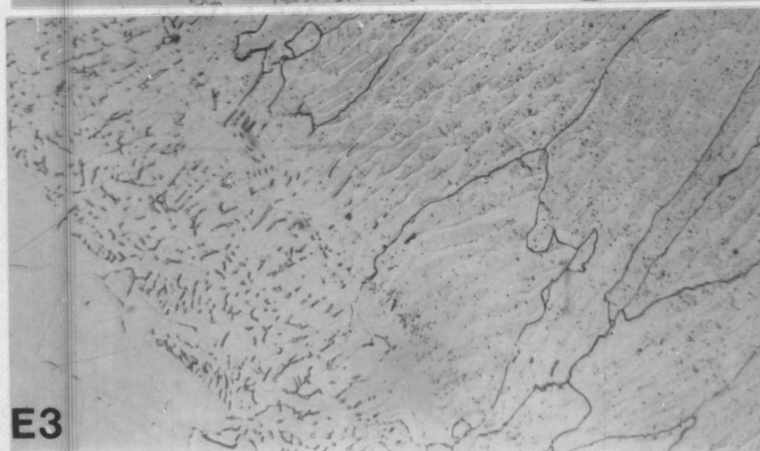
Figure 37. Microstructures of As-Deposited Fully Austenitic Stainless Steel Welds. (OLM, 200X)
