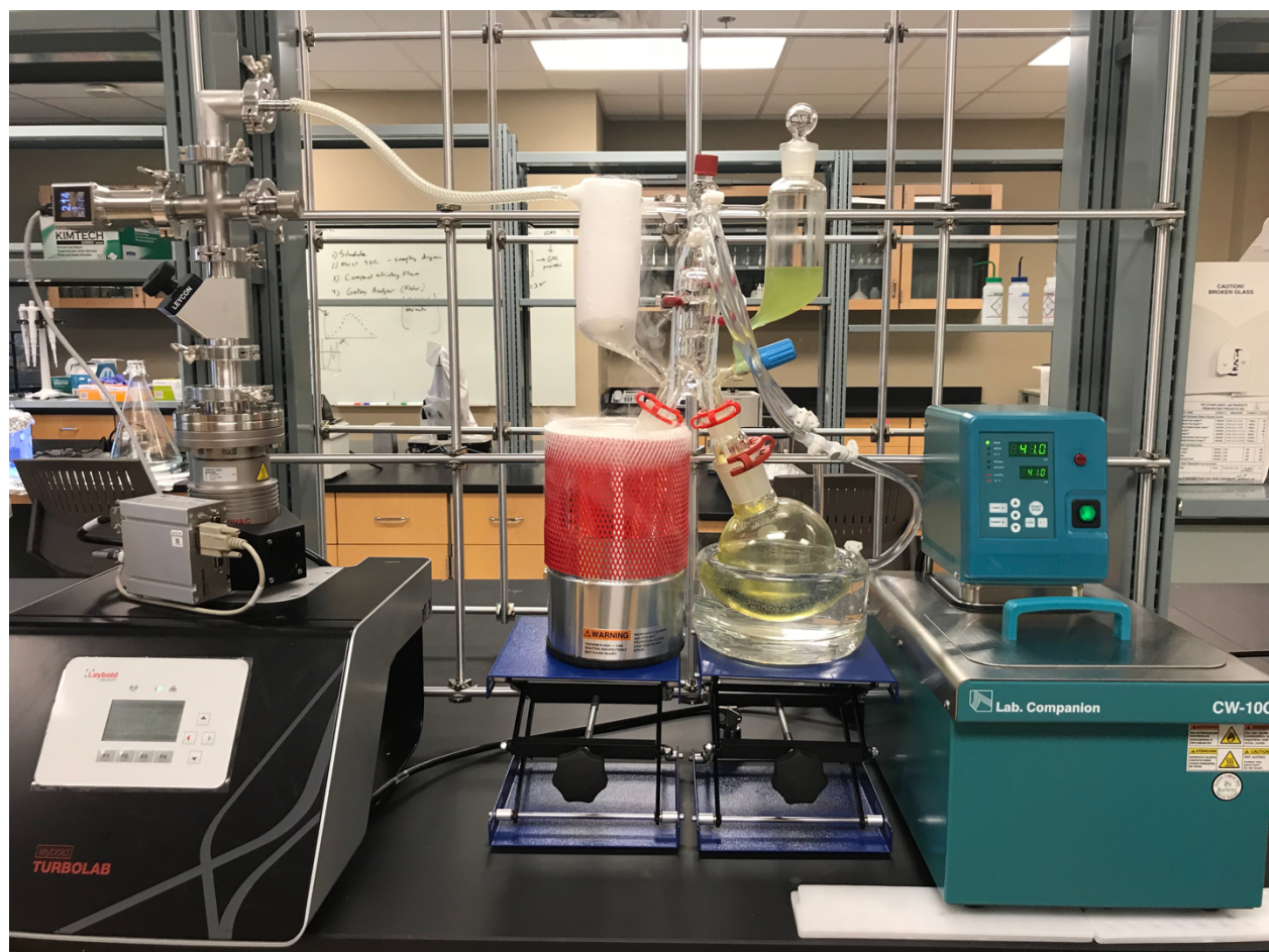
Figure 10: Solvent Assisted Flavor Evaporation Apparatus.
