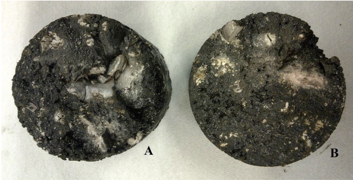
Figure 3.5. Example of the Aggregates damage. (A) Mixture One (307A), (B) Mixture two (307B)
