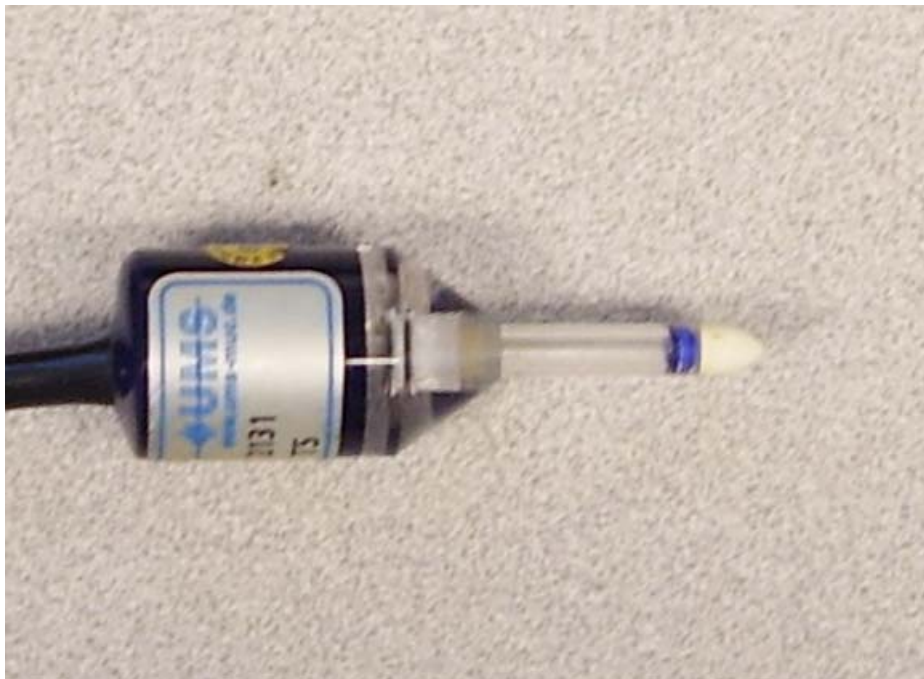
Decagon T5 Mini-Tensiometer
