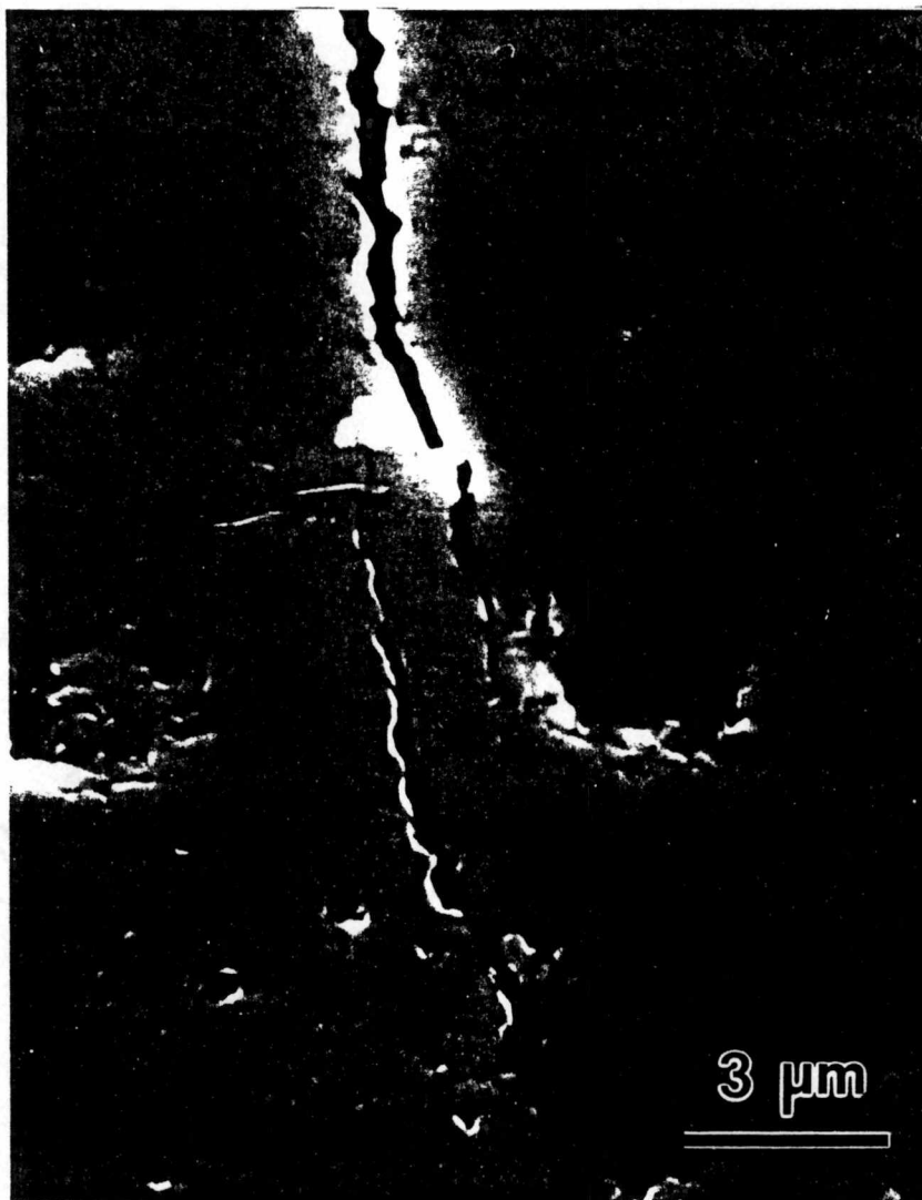
Figure 4.22 SEM micrograph shows a whisker debonded from the matrix as the result of the crack propagation.
