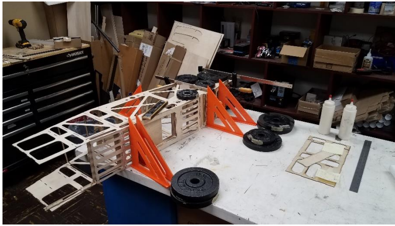
Figure 9.12: Drying of Fuselage after Applying Wood Glue
