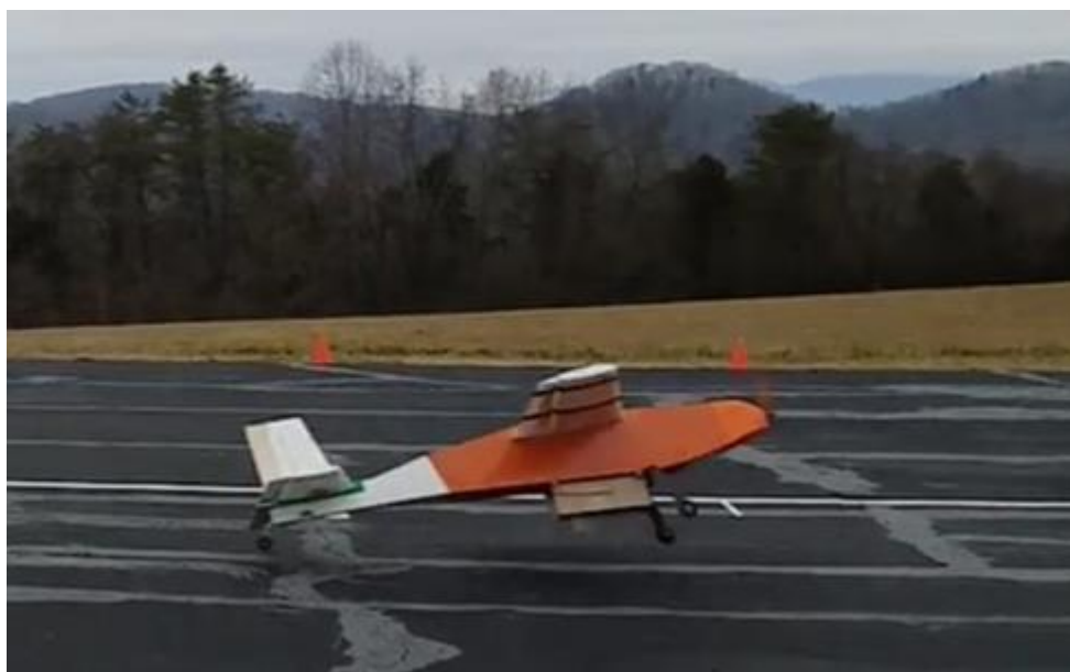
Figure 8.10: Photograph of airplane losing control immediately after takeoff with deployment mechanism attached.
