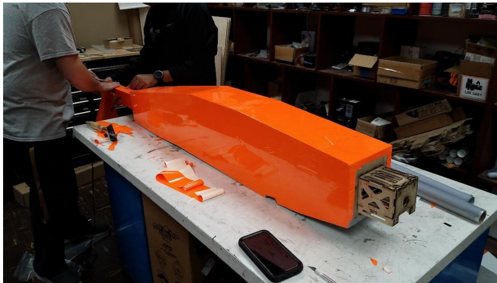
Figure 9.13: Covering the Fuselage with MonoKote
