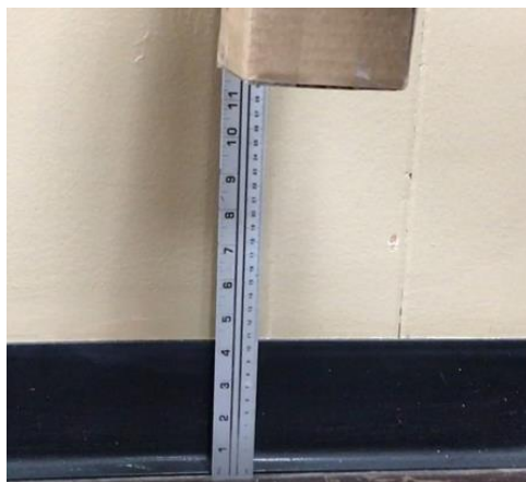
Figure 7.1: Sensor and cargo container during 10 inch drop test
