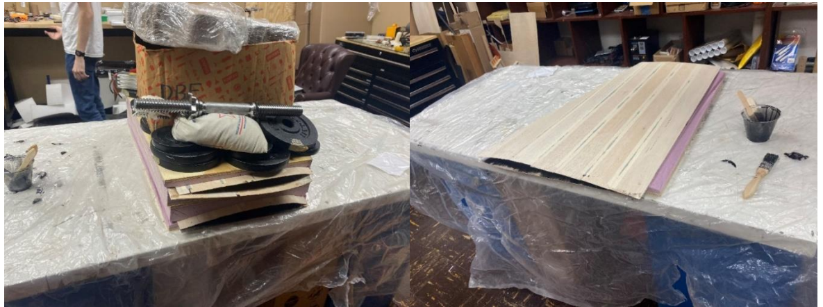
Figure 9.6: Skinning process for foam core wings.
