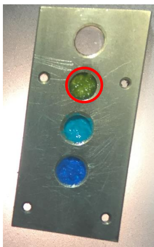
Figure 2.3. Photos of the samples of 2 for far-IR (Left) and Raman (Right) spectroscopic studies.
