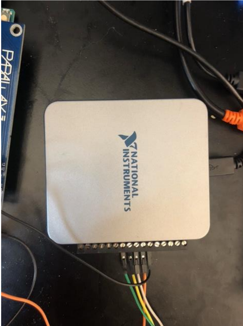
Figure 3-8: The DAQ model USB-6001 acted as the primary data collection device connecting the thermocouple readings to the development PC.
