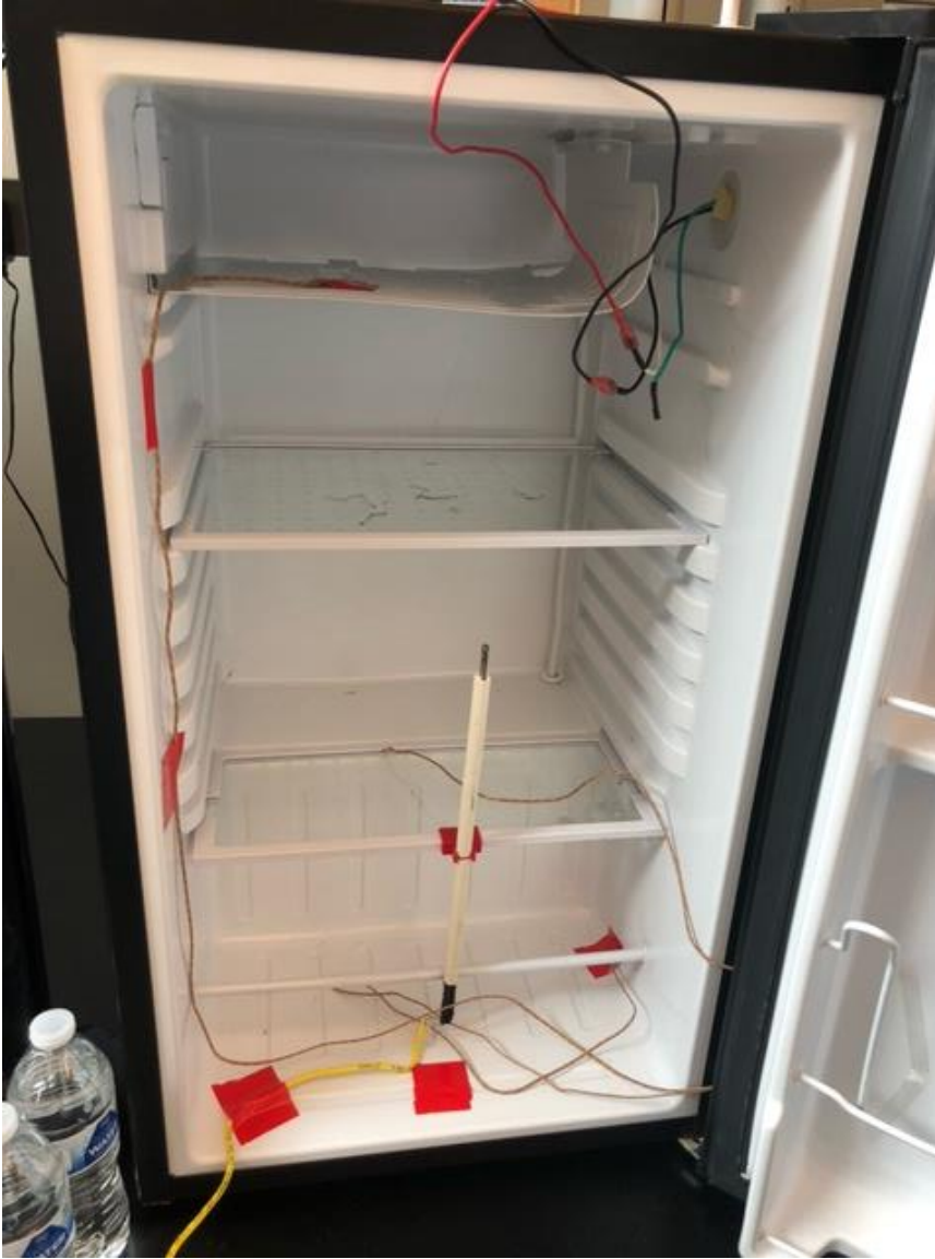
Figure 3-2: A look at the internal components of the platform to give a complete image of the system. This includes the thermocouples for tracking temperature and the wiring for compressor control.
