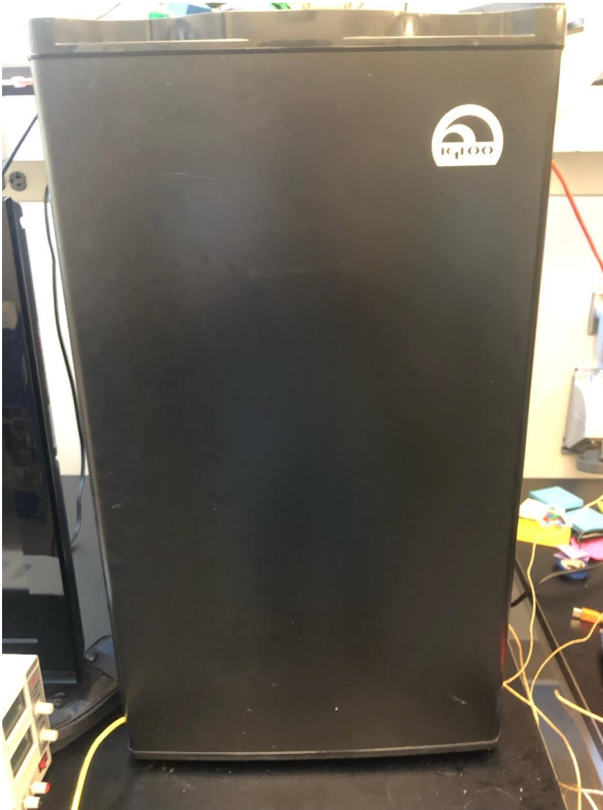
Figure 3-1: The main refrigeration platform was the FR3201, selected for its analog nature which made modifications easy, as well as its size, which balanced accurate scaling of thermodynamic modeling and accessibility due to weight.
