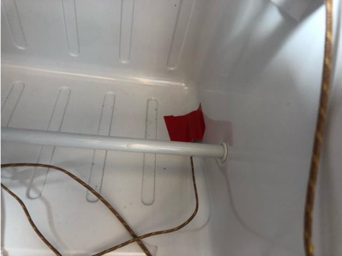
Figure 3-5: A surface thermocouple used to record temperature at the bottom of the refrigerator. While not directly used to influence system responses, these thermocouples helped to build an understanding of the system thermodynamics.
