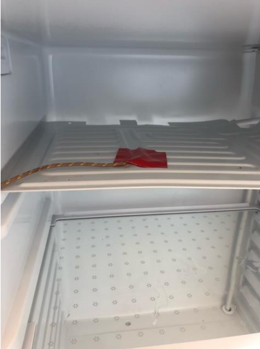
Figure 3-4: A surface thermocouple used to record the temperature of the evaporator. A great use for having additional thermocouples is error checking as the values of the thermocouple reads should be relatively close to one another.
