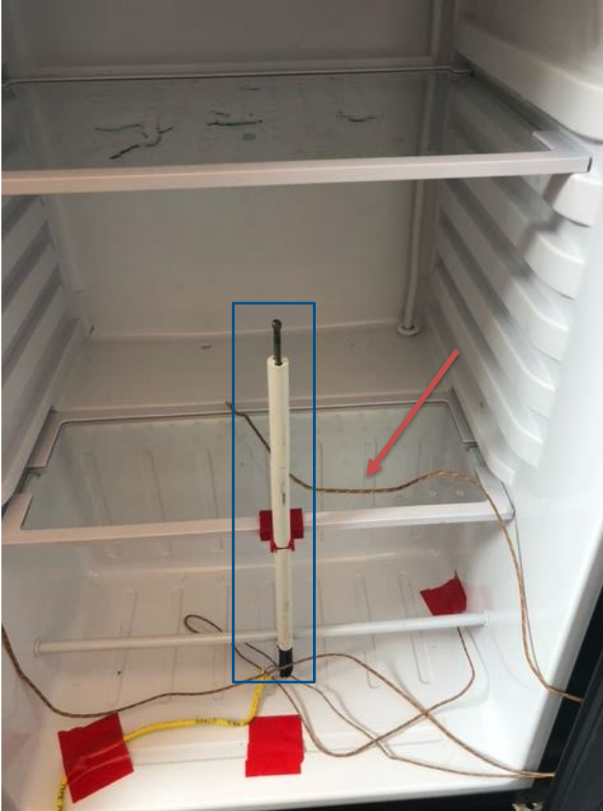
Figure 3-3: Highlighted in blue is the K type thermocouple for air temperature readings. This acted as the primary device that would determine system response. Pointed to with a red arrow is another K type thermocouple used for reading surface temperatures.
