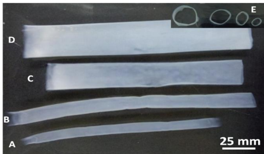
Figure 7.2: Photographs of BC-TS scaffolds synthesized on the inside surface (A) and on the outside surface (C) of 6.35 mm ID silicone tubes. Photographs of BC-TS scaffolds synthesized on the inside surface (B) and on the outside surface (D) of the 9.525 mm ID silicone tubes. Insert is the top view image (E) of the four sizes of BC-TS hydrogels synthesized using silicone tubes.
