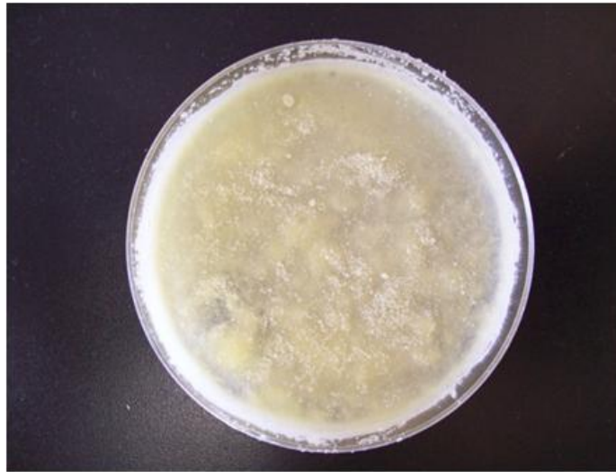
Figure 4.4: Photograph of porous BC culture consisting of Gluconacetobacter sucrofermentans and beeswax microspheres in Schramm-Hestrin Medium in a 100 mm diameter tissue culture dish. The beeswax microspheres floated in the bacterial medium during culture.
