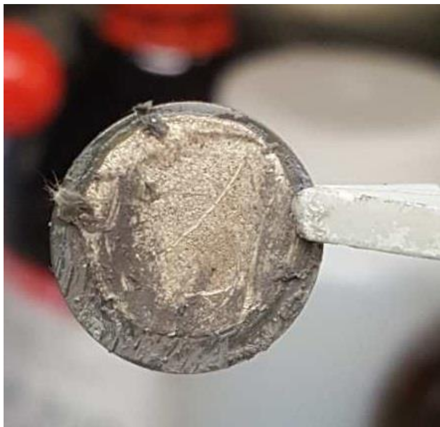
Figure 3.12 Photo images of the lithium metal disassembled from the Li/Li cell with PC doped PDMS- g -MPA Li + 10 /PEGMEMA 30 after galvanostatic cycling for 1100 hours at 0.04 mA/cm 2
