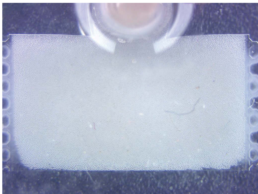
Figure 25. Microscopic picture of AG-50X8 1 day after adding the ^{225}\text{Ac} .
