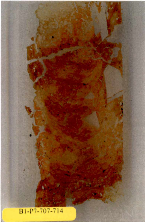
707-714 cm depth, Soil horizon Cr Gravelly sandy clay. Prominent features include many deeply weathered sandstone lithorelicts, zones of silt infillings and redox. mottling.
