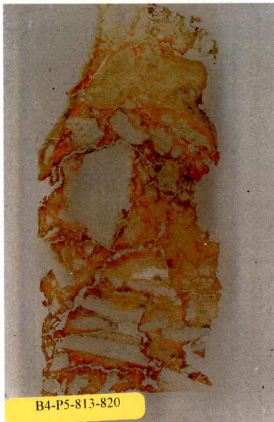
813-820 cm depth, Soil horizon Bt8 Gravelly clay Significant RF's that include deeply weathered shale lithorelicts and Mascot-like dolostone, some pores/grains/shale lithorelicts coated w/ kaolinitic cement, ped. clay coats, and thick Fe-oxide coats.
