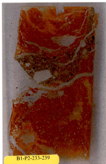
233-239 cm depth Highly oxidized clay with loamy interbed possibly representing surficial (A or BE) sandy loam infillings within a decayed root pore.
