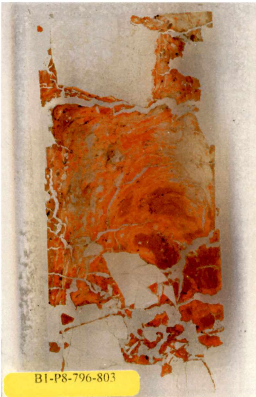
796-803 cm depth, Soil horizon Bt6 Gravelly silty clay. All RF and sand grains are angular. Heavily mottled and convoluted bands of multigenerational pedogenic clays and Fe- oxide coats. Angular ped. clay papules and vfg -sandstone lithorelicts.
