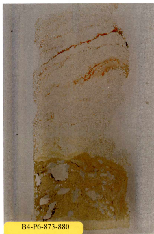
873-880 cm depth, Soil horizon Bt10 + Bt11 Clayey sand Overall greener, drab coloration of clays, sands are med.-coarse grained, moderately to well-sorted, and well-rounded, sharp contact b/w Bt10 and Bt11 (gravelly clay).
