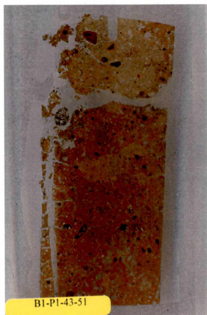
43-51 cm depth Thin-section showing gradational boundary between BE and Bt1 soil horizons. Note common, large multigenerational Fe-oxide concretions.
