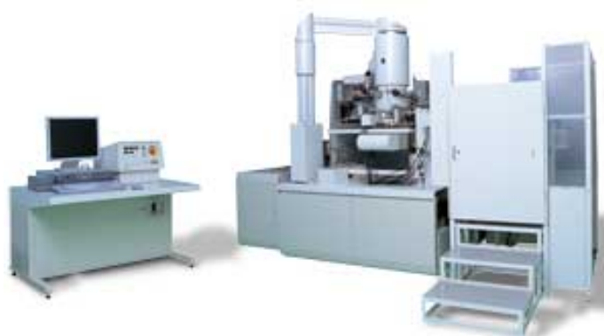
Figure 1-8. Picture of the JEOL JBX 9300FS Electron Beam Lithography system similar to the EBL tool located at CNMS.
