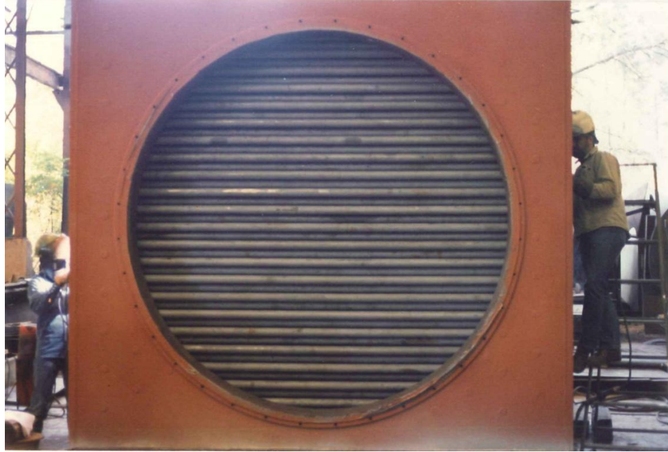
Figure 3 - The Inlet of H2's Cross Flow, Staggered Tube Heat Exchanger
