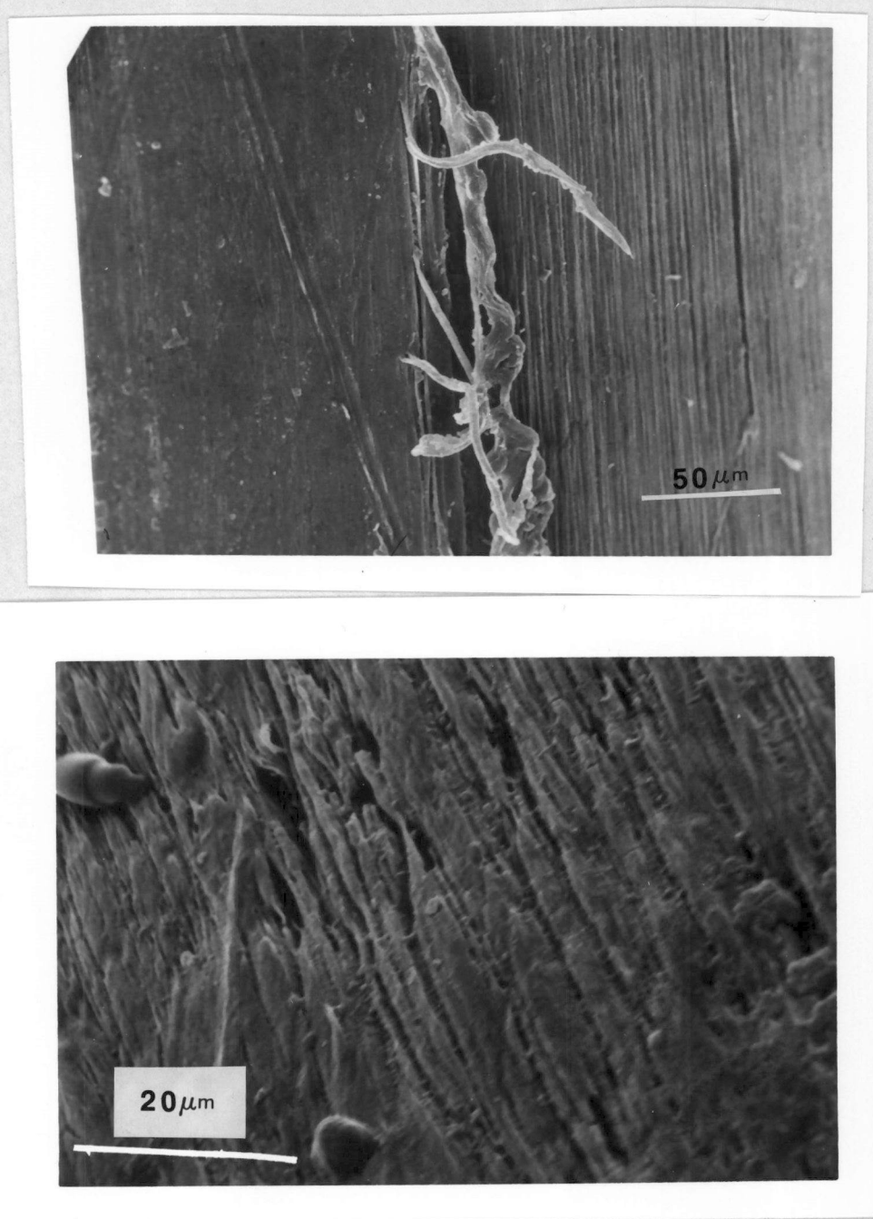
Figure 28. SEM micrographs showing the surface structure of (a) natural drawn, (b) superdrawn samples.
