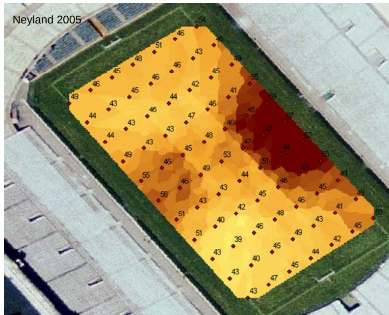
Figure 5. 2004 and 2005 post season interpolation of Clegg hammer data using the kriging method taken of Shields-Watkins field in Neyland Stadium, Knoxville, Tenn.
