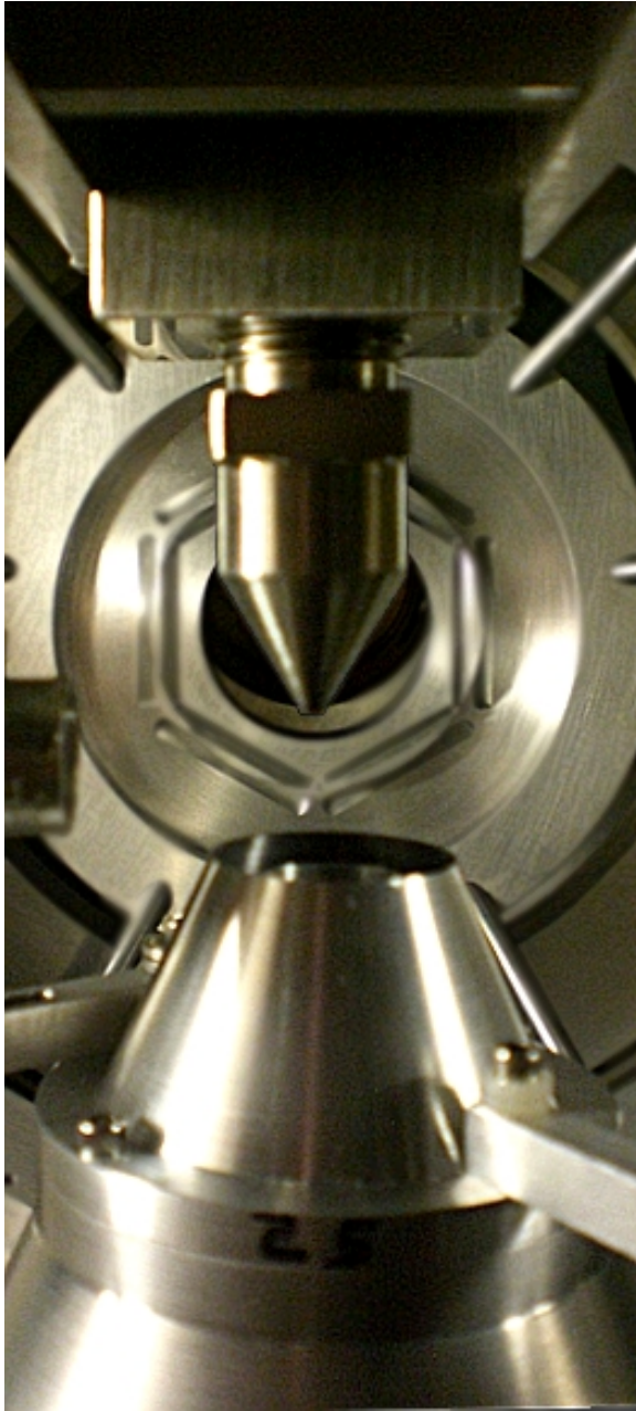
(a) Photograph of inside the JENSA chamber showing a nozzle and two concentric receivers. When the system is operational, gas leaves the nozzle through the gap and is collected in the concentric receivers. The collected gas is then recirculated back into the compressor is reused as target gas. Photograph courtesy of Kelly Chipps.
