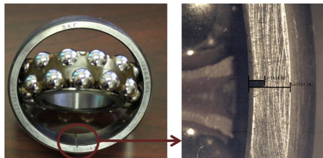
Figure 3-6 SKF 1205 ETN9 with a seeded fault
