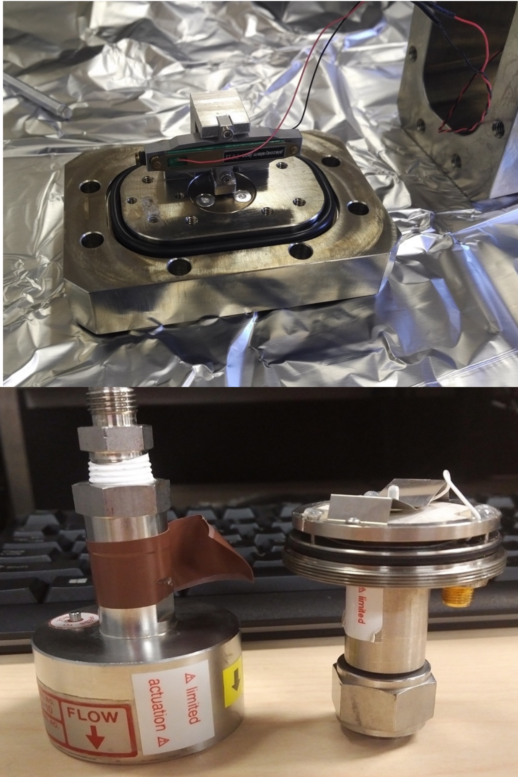
Figure 3.5. The difference between the UW-M (top) and PV-10 (bottom) piezos and valve sealing mechanism.
