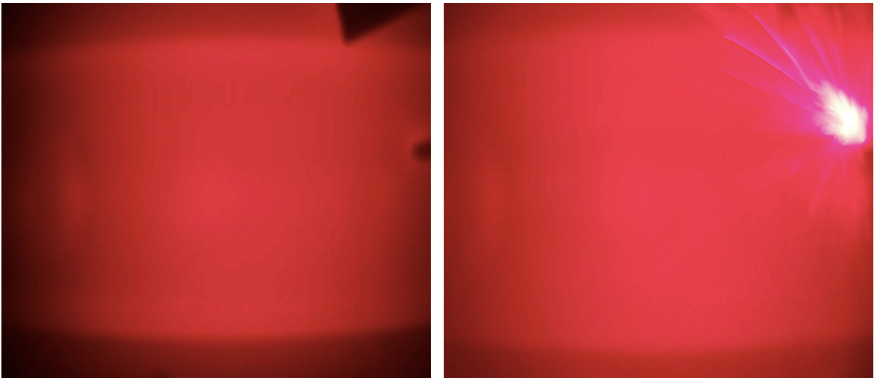
Figure 1.4. Helicon only plasma with DLP inserted (left) and the destruction of the DLP during microwave injection (right).
