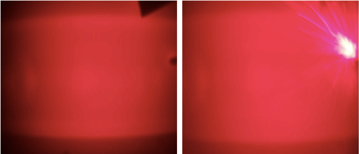
Figure 2.4 Destruction of a DLP during microwave injection
