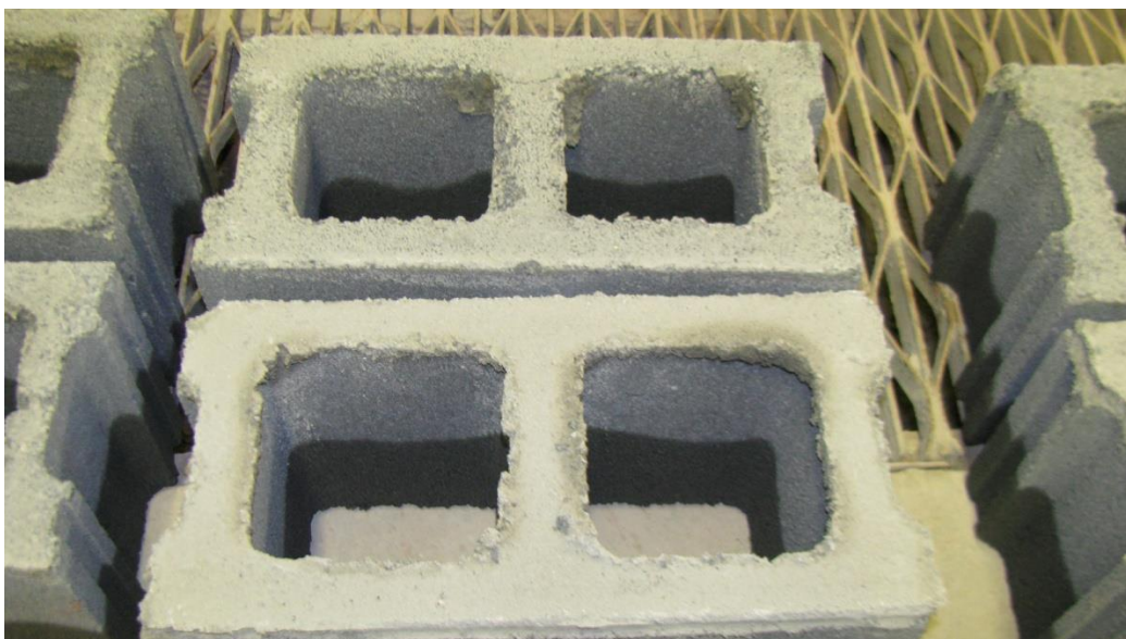
Figure 11.3—View of Freshly Broken Joint
