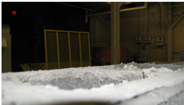
Figure 11.12—Broken Joint Surface Roughness
