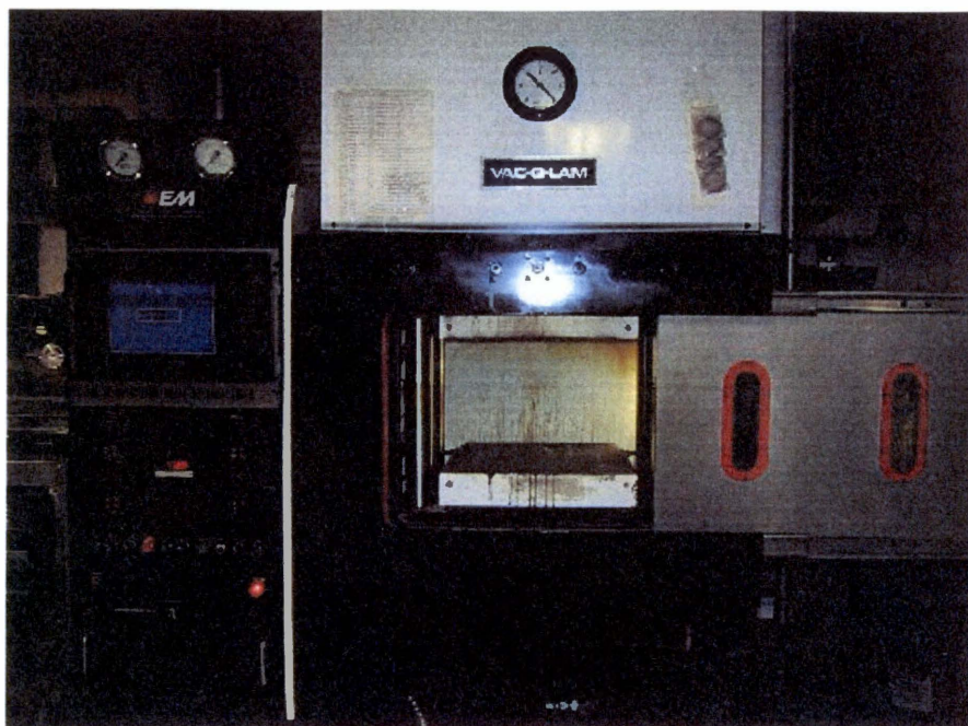
Figure 2.1 OEM composite curing system
