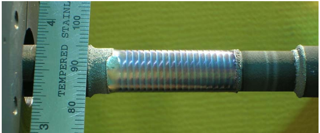
Figure 4.3.3(a) A 30 mm long and 0.3 mm thick W-TiC deposit made on a graphite mandrel by laser processing a 0.6 mm W-TiC barrier coating induction hardened for 5 hours. Laser processing was done at 1500 W.
