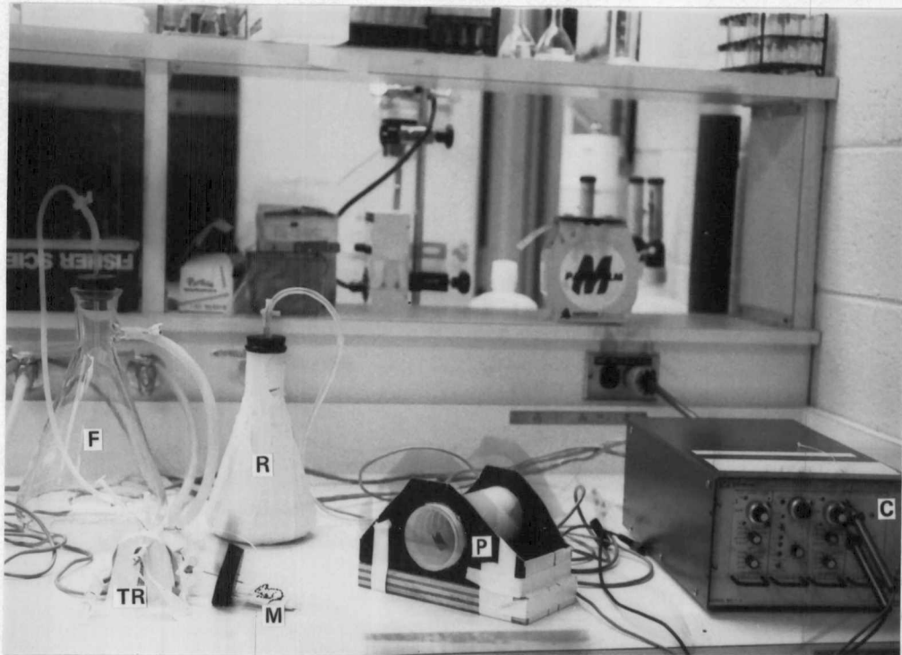
Figure 11. Apparatus for lung function studies. P = plethysmograph, C = carrier demodulator, M = mouse in supine position, R = reference volume flask with copper wire, and insulated to provide constant reference pressure, F = flask, to prevent pressure fluctuations, and TR = transducer.
