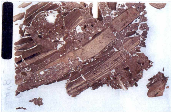
24-27 cm depth, BC horizon, shale/siltstone saprorelicts.
