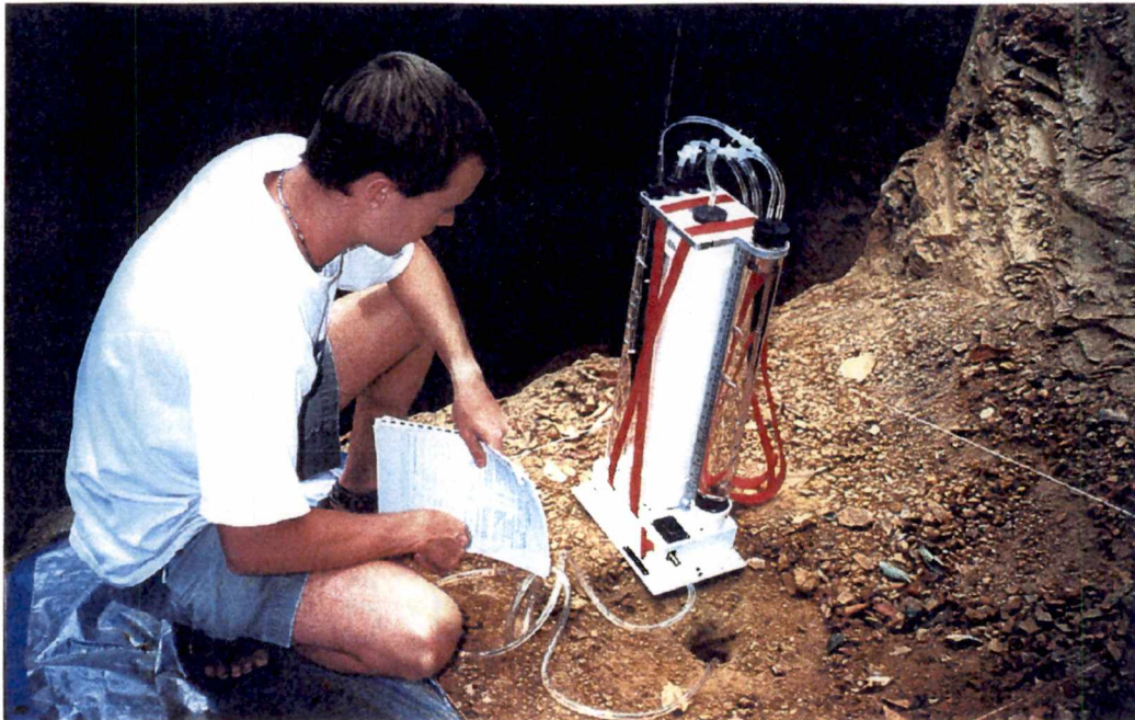
Typical CCHP set up during field measurements.
