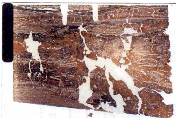
205-208 cm depth, C2 horizon, ribbon limestone saprolite with some silt lenses.
