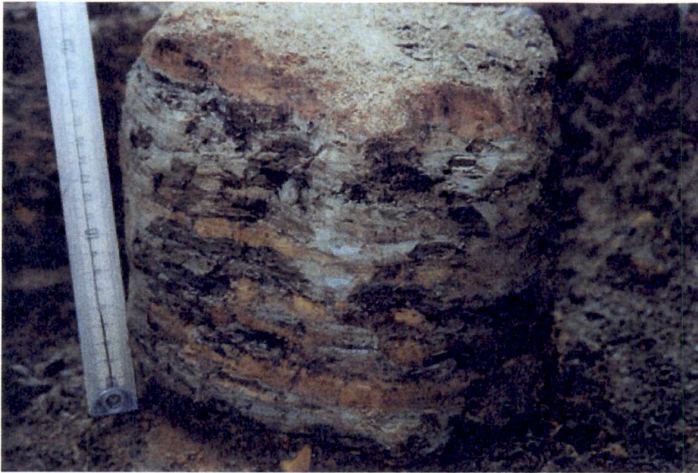
Typical column excavated to be cut down and later sent off to be thin sectioned.
