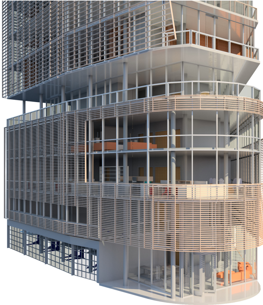
Figure 20: Building is completed with ceramic screen
