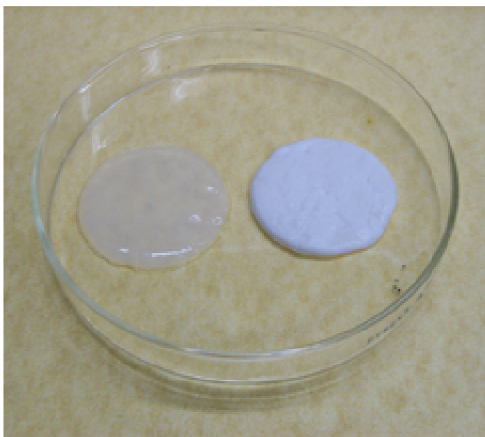
Figure 4.1: Comparison of unaltered bacterial cellulose (left) and cellulose after three incubation cycles in 100 mM \text{CaCl}_2 and 60 mM \text{Na}_2\text{HPO}_4 (right)
