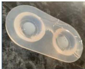
Figure B10. Heated ballistics gel in the iTrainer eye mold.
