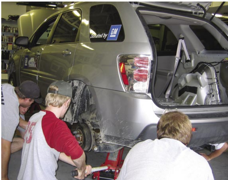
Mechanical engineering students begin modifications to the drivetrain of the 2005 Chevrolet Equinox which will be transformed into a hybrid electric vehicle with funding from DOE's Challenge X competition.
