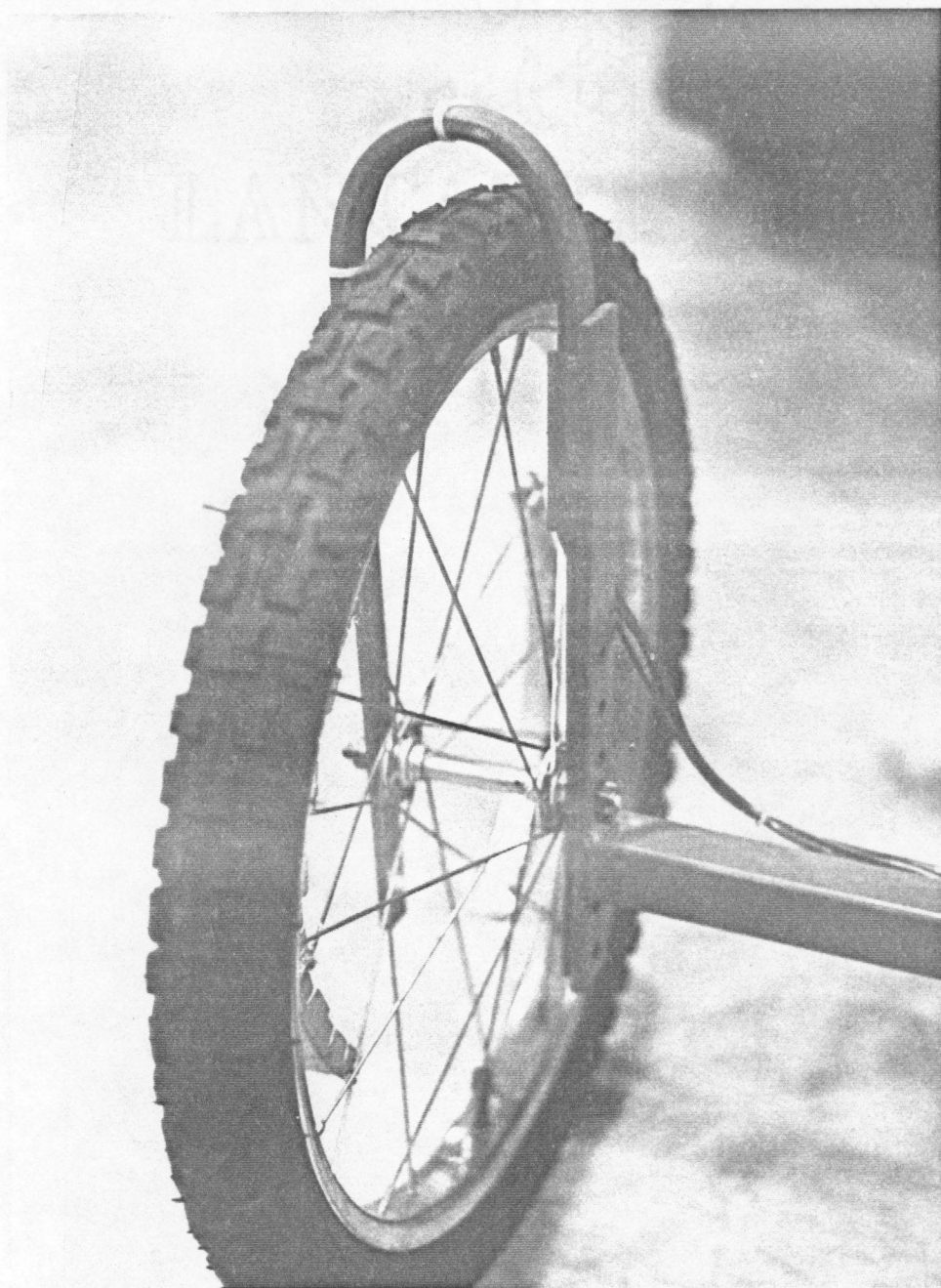
Figure 4. Ground wheel used to maintain proper nozzle height on the experimental chemical applicator.
