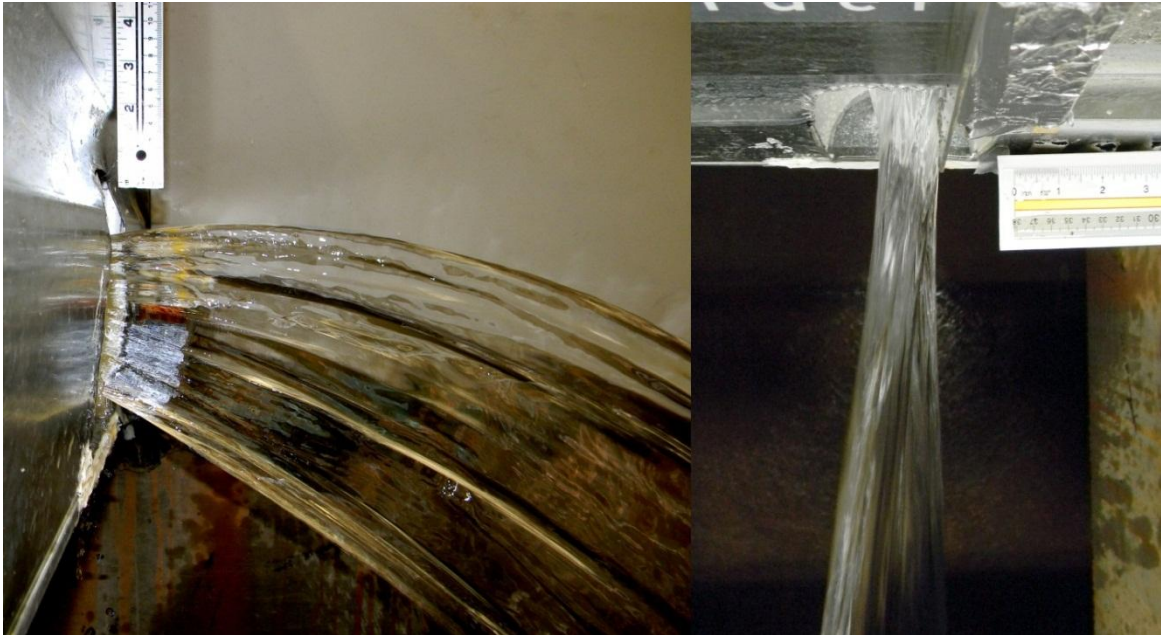
Figure 13. Vena contracta visual assessment, D = 10.2 cm and d = 7.62 cm. The width of the jet was 3.07cm and the height was 10.6cm at a distance 5.1cm from the orifice
