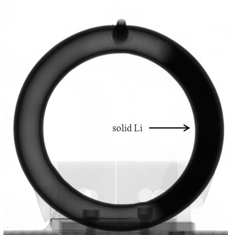
Fig. 7: Torus Mo-Li heat pipe at ambient conditions on CG-1D [Ref. 38].
