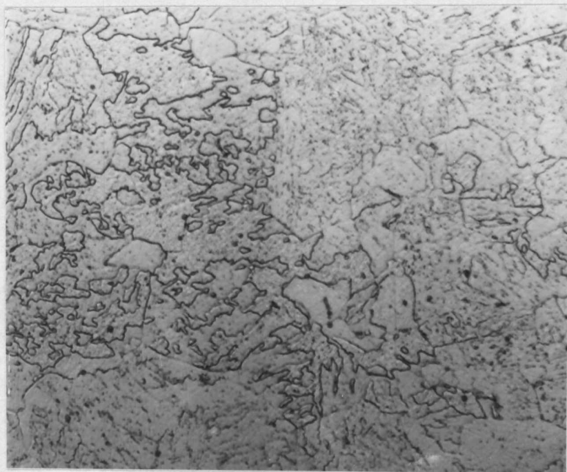
Figure 40. Light micrograph of ESW weld metal after 1500 hours at 1050 F showing bainitic structure. Polished and etched with 2% nital. 250X.
