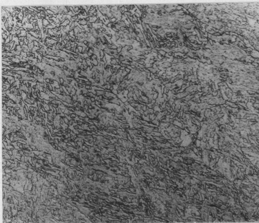
A. Light micrograph, showing bainitic structure. Polished and etched with 2% nital. 250X.
