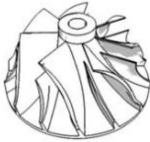
Figure 3.9 Turbine wheel of dimensions 54 x 54 x 28 mm, volume 20,618 mm 3 , 2012 (Baumers et al.)
