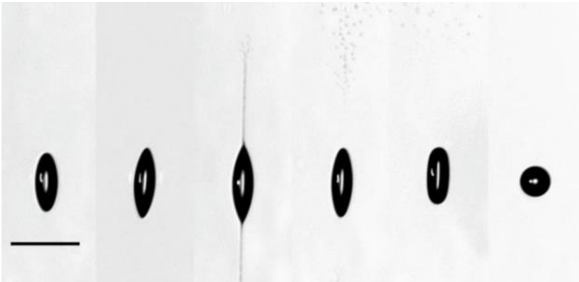
Figure 11: Evolution of transient cone-jets on levitated ethylene-glycol droplet [51].
