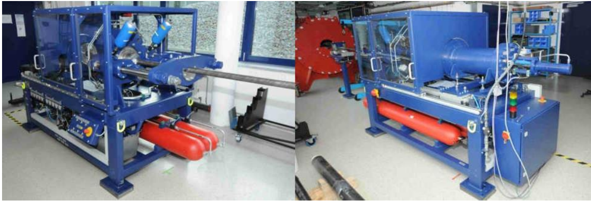
Fig. 45 Pressurized gas gun with 30 mm smooth bore barrel.
