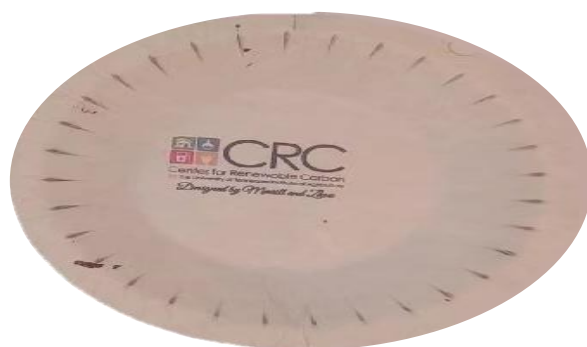
Figure 7.13 Molded plate-shaped sandwich-structured paper composite with a printed Center for Renewable Carbon (CRC) logo.
