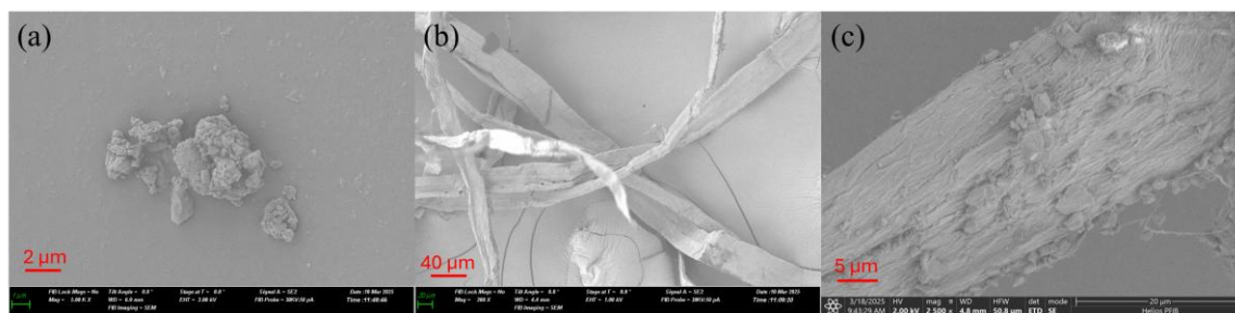
Figure 8.10 Scanning electron microscopy (SEM) images of (a) lignin micro/nanoparticles (LMNPs) and (b) pulp fibers, (c) LMNP attached to pulp fiber surface before hot press.
