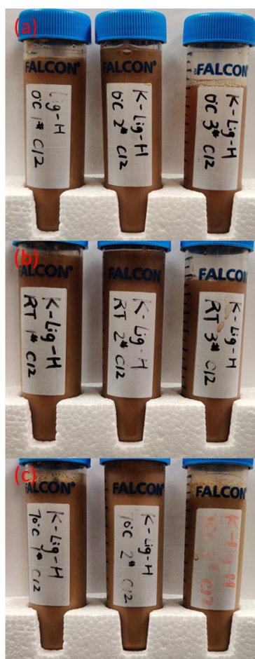
Figure 4.3. Photographs of LMNP suspensions after 90 days of incubation at 4 °C, prepared by 12 UFG (ultrafine friction grinding) passes at (a) 0 °C, (b) 25 °C and (c) 70 °C.
