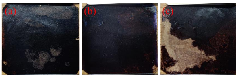
Figure 6.14 photos of LMNP paper composite with the different water content of lignin suspension before the hot press, (a) C40-P3-T160-M10, (b) C40-P3-T160-M30, (c) C40-P3-T160-M50
