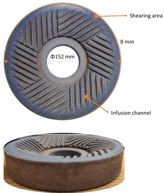
Figure 5.1 Photographic representation of the grinding disks of the ultrafine friction grinder
