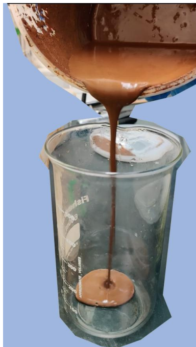
Figure 5.2 Photographic depiction of water based LMNP suspension produced at 25 °C, 40 wt. %.
