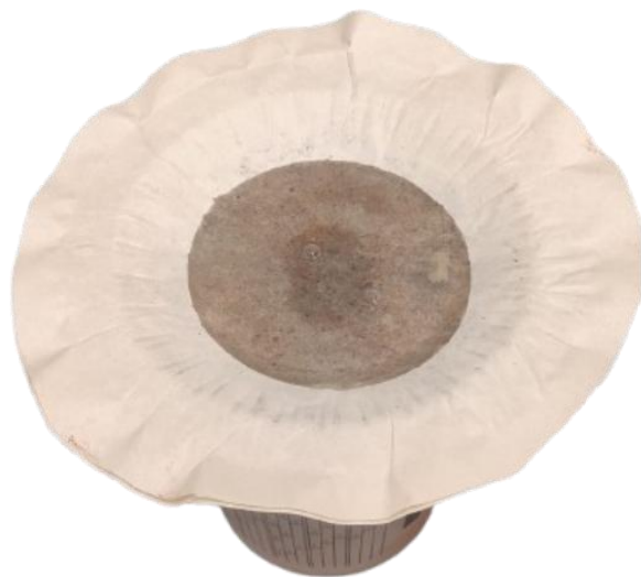
Figure 7.12 Molded plate-shaped sandwich-structured paper composite retaining vegetable oil for over 1 hour without leakage.
