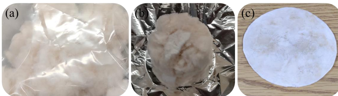
Figure 8.2 (a) Individual pulp fibers in their raw form, (b) fiber assembly before hot pressing, and (c) final product of L0-PF10 after hot pressing.
