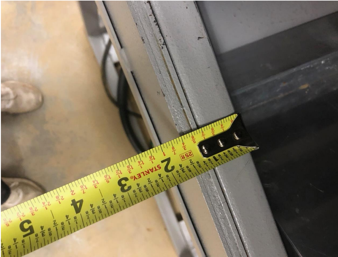
Figure 17. Measurement of the sandwiched lead shielding in the X-ray cabinet before modification. \frac{1}{8} in. of steel, \frac{1}{4} in. of lead, and another \frac{1}{8} inch of steel are shown. The 1 in. steel piece at the end of the tape measure is a structural steel tube.
