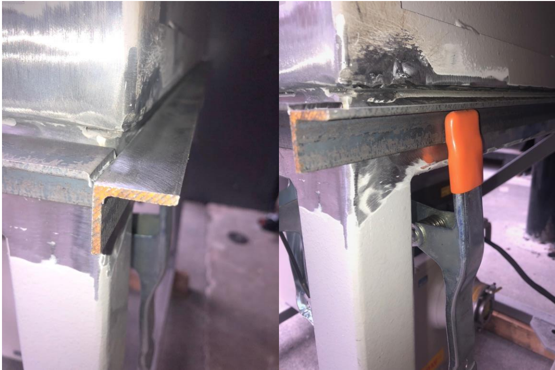
Figure 22. Image of 1 in. angle iron being fixtured with clamps on each face before welding.
