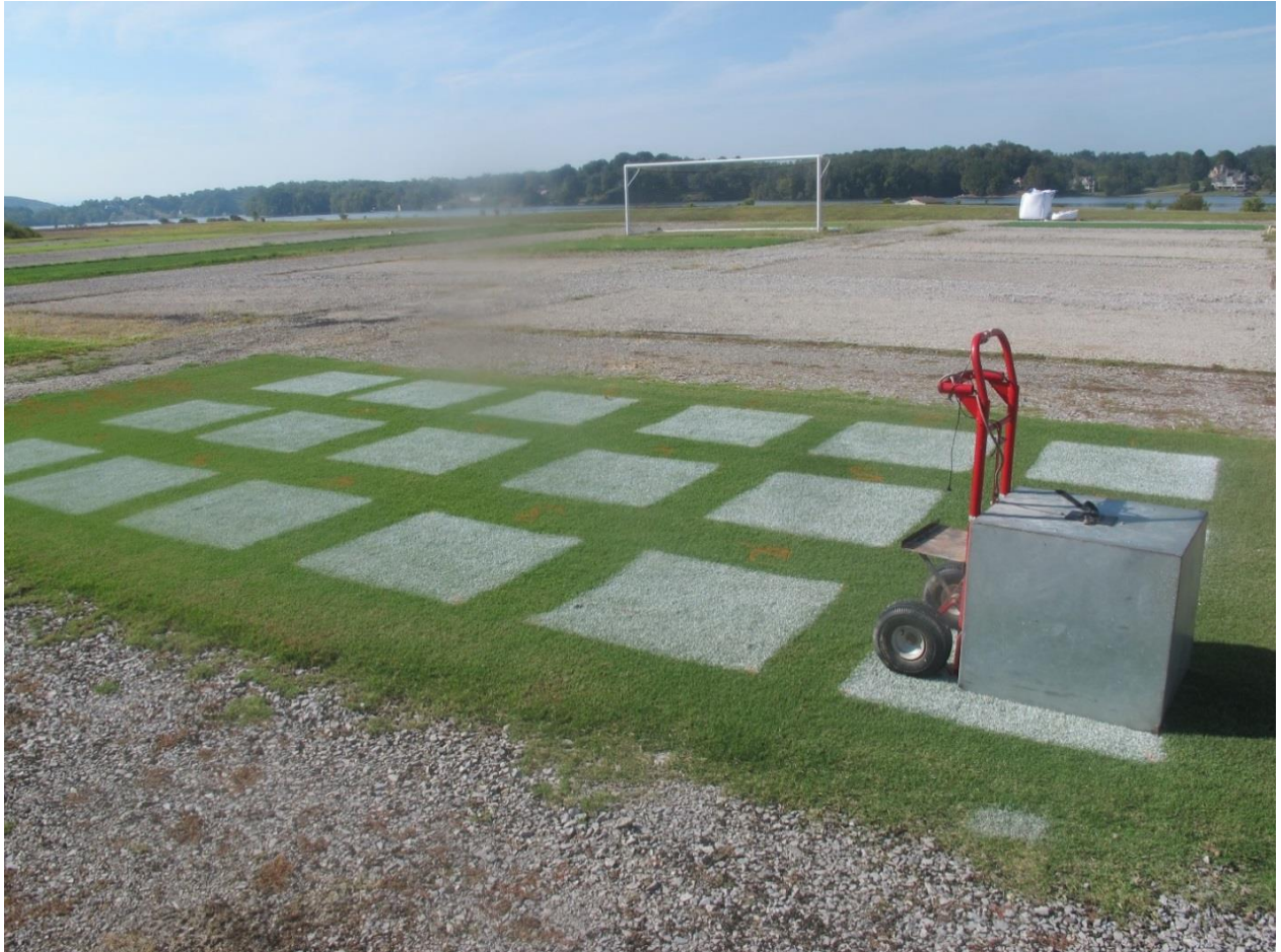
Figure 9. Illustration of digital image analysis photograph capturing using the light box on different athletic field paint treatment areas, 2019. University of Tennessee, Knoxville, TN.
