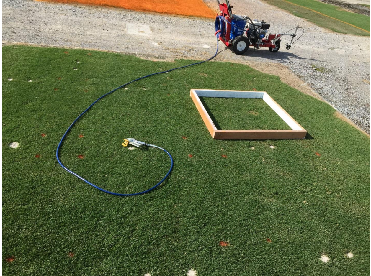
Figure 1. Pioneer Brite Striper 3000 paint machine loaded with Pioneer Brite Stripe white paint mixed at a 1:1 paint and water ratio. Wooden stencil measuring 0.91 m x 0.91 m in size, with a 0.3 m buffer zone, applied to hybrid bermudagrass [ 'Tifway' Cynodon dactylon (L.) Pers. x Cynodon transvaalensis , Burt-Davy] turfgrass, 2015. University of Tennessee, Knoxville, TN.
