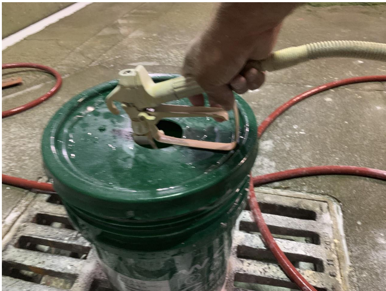
Figure 4. Calibration of different treatments of athletic field paint using Pioneer Brite Striper 3000 paint machine loaded with Pioneer Brite Stripe white paint mixed at a 1:1 paint and water ratio, 2016. University of Tennessee, Knoxville, TN.
