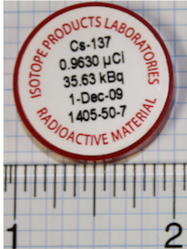
Figure 3.4: Calibration source used for spectrometer energy and efficiency calibrations.
