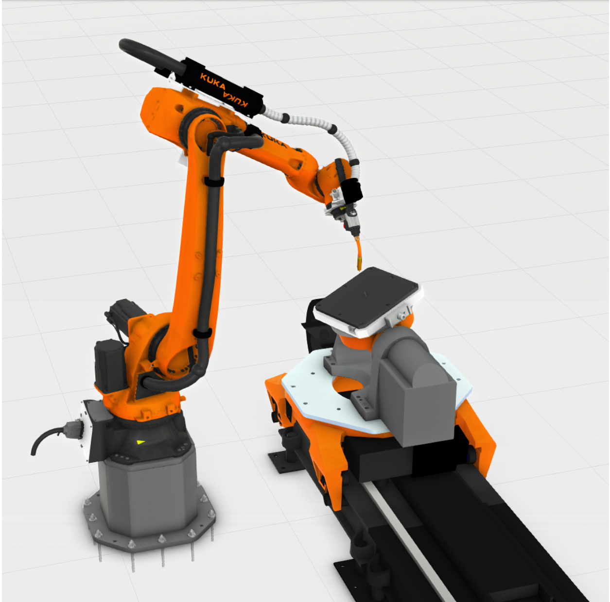
Figure 2.4: Robot manipulator and part positioner in Octopuz simulation
