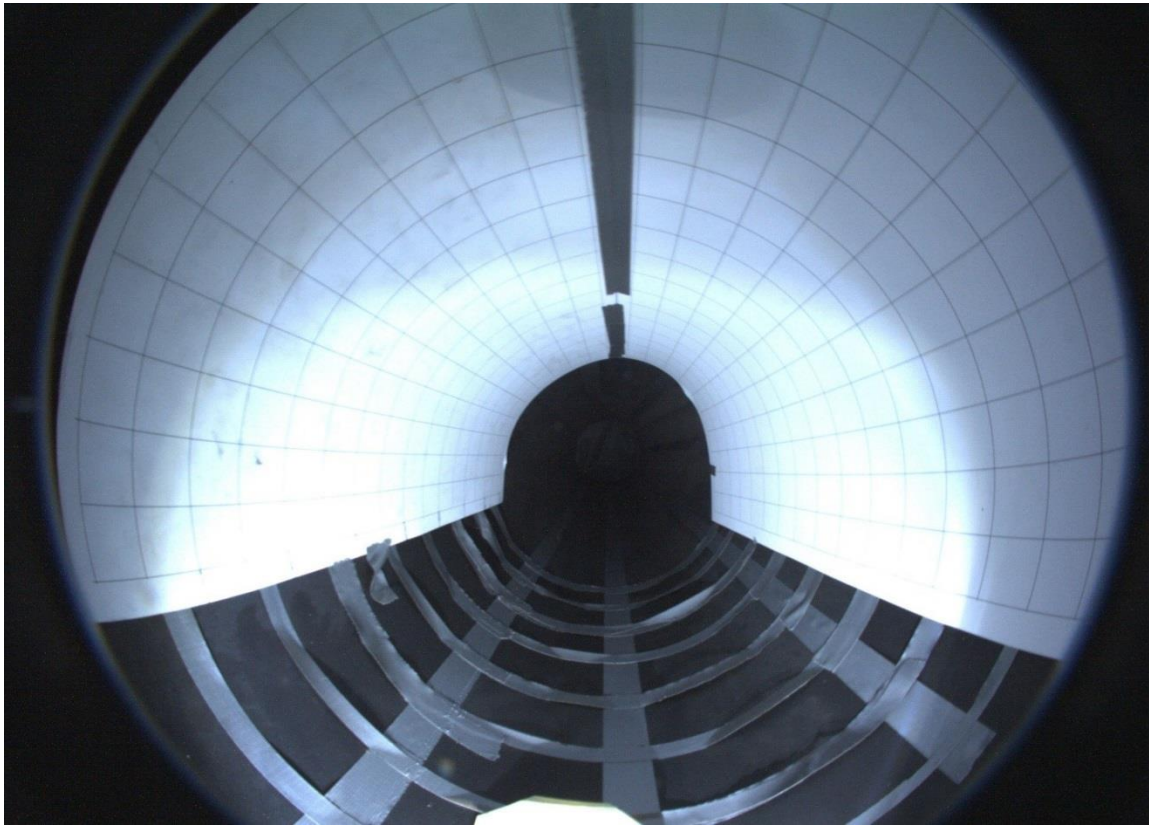
Figure 2: Image taken by the fisheye camera of the grid placed inside the pipe.
