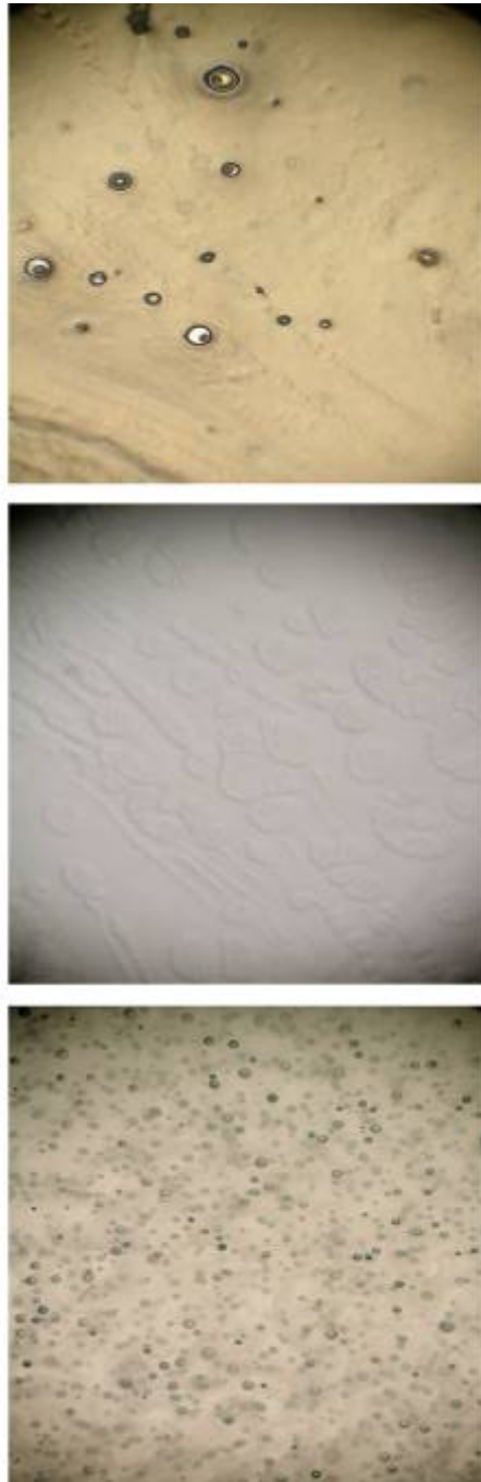
Figure 18 - Air bubbles trapped during encapsulation (top to bottom: EP42HT-2, EP30MED. EP21LV)
