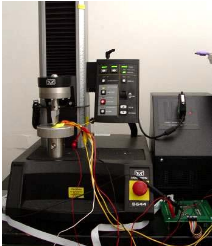
Figure 20 – Experiment setup of the encapsulated microcantilever with Instron tensile machine
