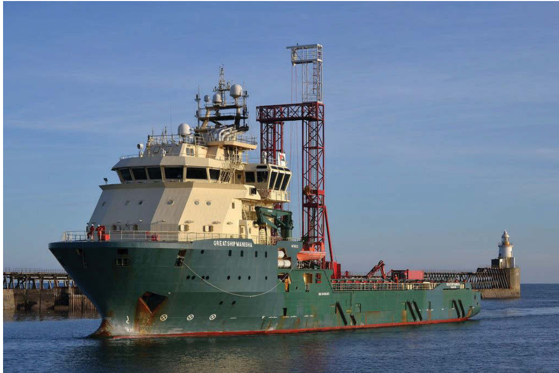
Figure 1.2: The R/V Greatship Manisha is the mission specific retrofitted drilling platform that was used to collect rock and sediment samples during IODP Expedition 347.
