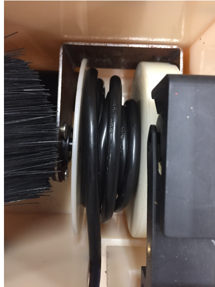
Figure 26: Power Cord Diameter Failure
