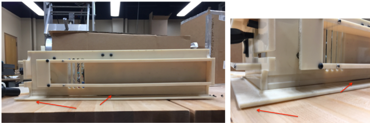
Figure 22: Bottom Plate Failure
