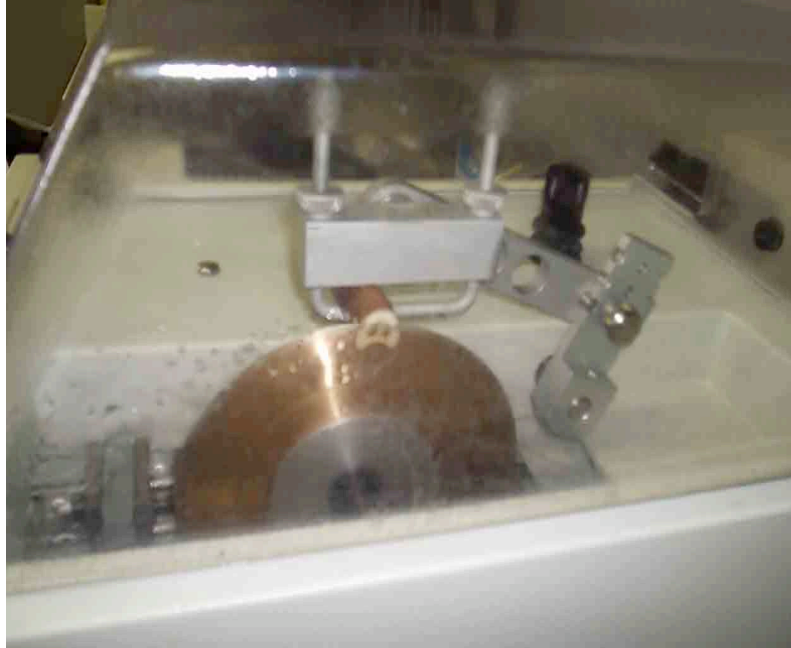
Figure 17: Buehler 1000 Isomet saw cutting 0.08mm section from shaft of bone.
