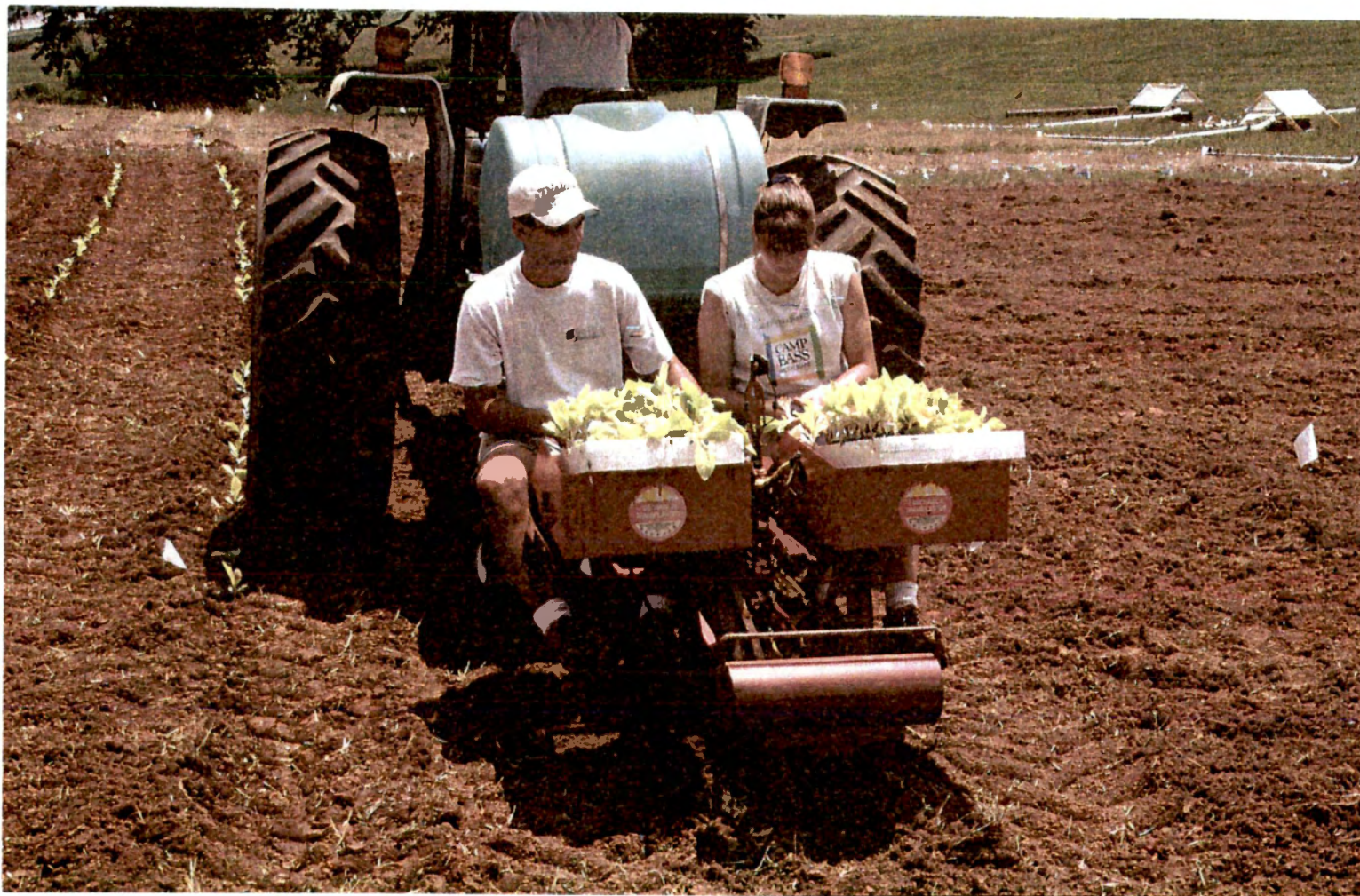
Plate 3. Photograph of no-till transplanter in use.
