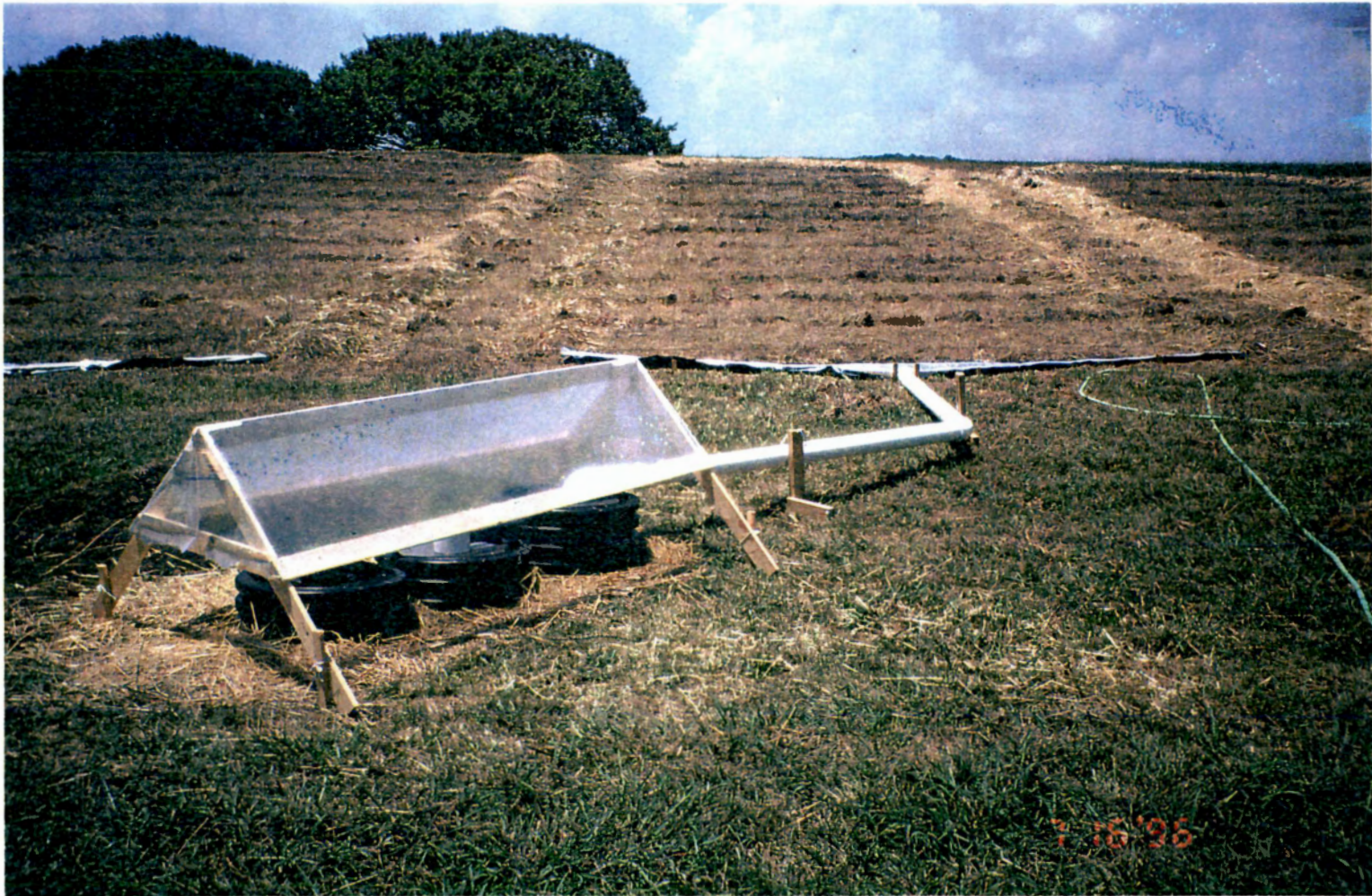
Plate 5. Photograph of collection buckets, sumps, and A-frame teepee cover.
