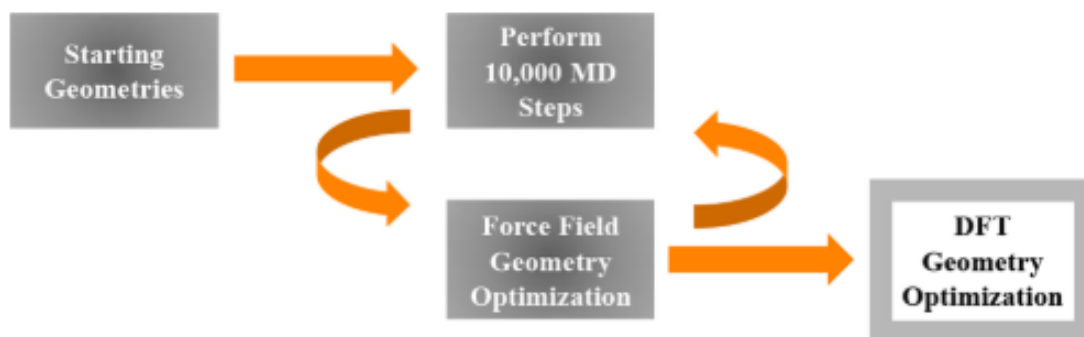
Figure 1.4: A flowchart examining a strategy to remove expert bias from conformational searches. Molecular dynamics simulations can be used to generate conformations which are optimized by DFT to find global minima on the potential energy surface.
