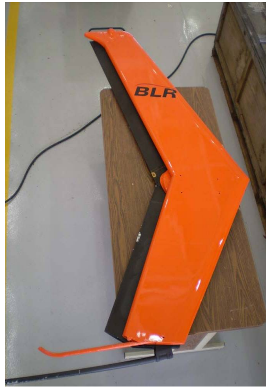
Figure 5. Comparison of Modified OH-58D Fin (orange) to Original Fin
