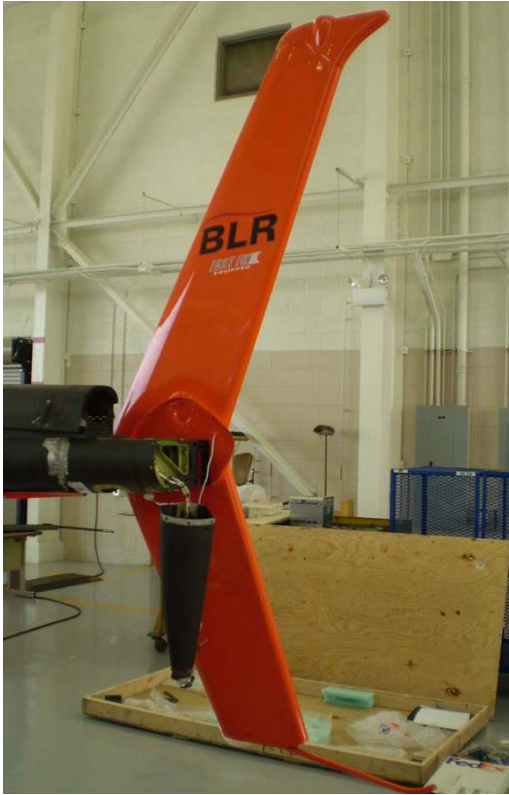
Figure 5. Comparison of Modified OH-58D Fin (orange) to Original Fin
