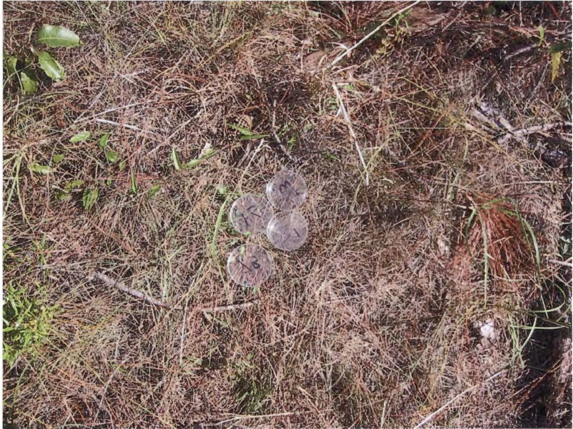
Figure 4.1 Photograph of air-fall charcoal traps in use. Each trap consisted of the tops and bottoms of two plastic petri dishes coated on the bottom (inside) with petrolatum. Photograph by D. West.
